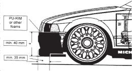
more than 10mm. If an opening is created through the foam bumper for cooling air, the combined thickness of the foam (above and below the cooling hole/slot) must still be a minimum of 40mm in height.
