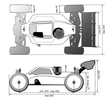
Wheel overall diameter must be between 109 and 120 mm. Wheel overall width 47 mm maximum.
