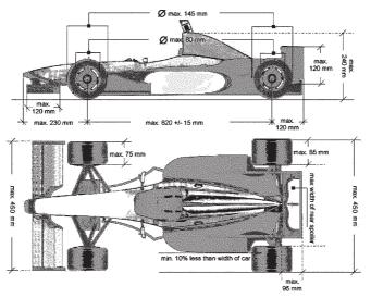
The rear wing must fit into a side profile box of 95x120 mm. The number of added wings inside is free. The rear wing must not be wider than the space between the rear tyres.
