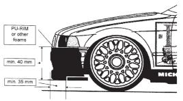
foams, that are used in 1:1 car construction to absorb impact energy. At no point may any part of inflexible material for bodyshell mounting protrude from the body more than 10mm.
