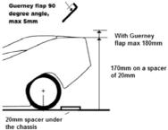
267 mm 170 mm (on 20 mm blocs) urney strip 180 mm.(on 20 mm blocs) 100.00 mm, 110 mm for 2wd & flat chassis cars
