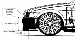
foams, that are used in 1:1 car construction to absorb impact energy. At no point may any part of inflexible material for bodyshell mounting protrude from the body more than 10mm.
