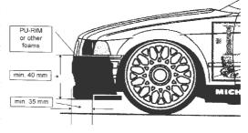
1:1 car construction to absorb impact energy.
