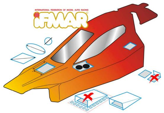
If no "marked" air scoops/vents are designed in the original mould to assist airflow to the motor or ESC, then material may be removed to a maximum of 10 mm in any given direction within a maximum square area of size 30 mm x 30 mm, in two places only. Windows are not allowed to be removed or include holes, other than for the purpose of the antenna.
