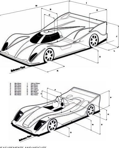
6.2 MEASUREMENTS AND WEIGHTS Rectangle max 52 x 26 mm Maximum overall width of the car: 172 mm (Excluding shell) Minimum weight: 730 grams. Wing: Maximum width: 172 mm, the wing profile has to fit in a rectangle of 52mm (height) x 26mm Spoilers: Max. Spoiler height: 25 mm, max length 35 mm. These dimensions include the
