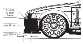
1:1 car construction to absorb impact energy.
