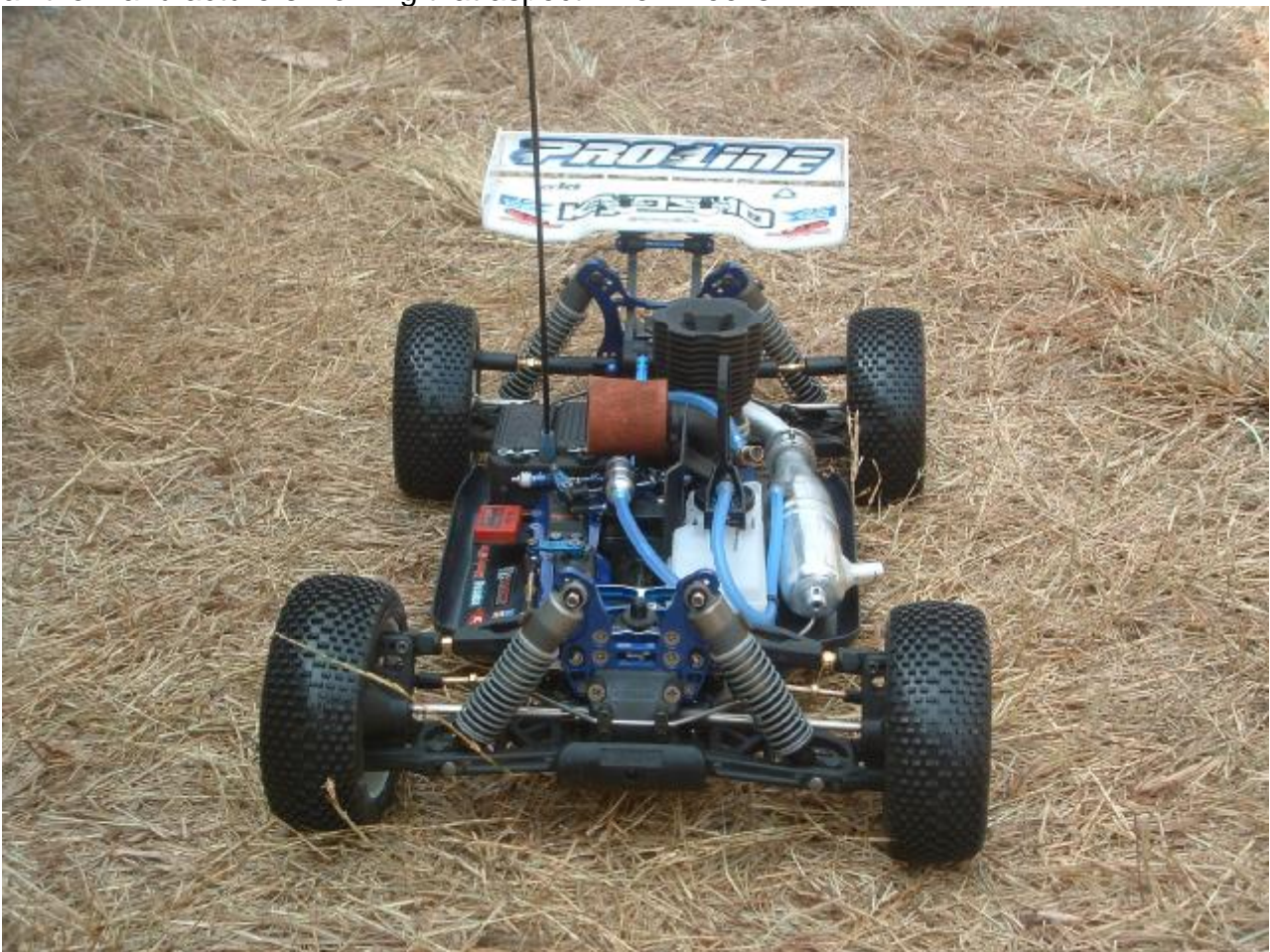
Mark Pavidis car, Proline wing, OS engine with magnesium head and the tyre of the race, Proline Crime Fighter
